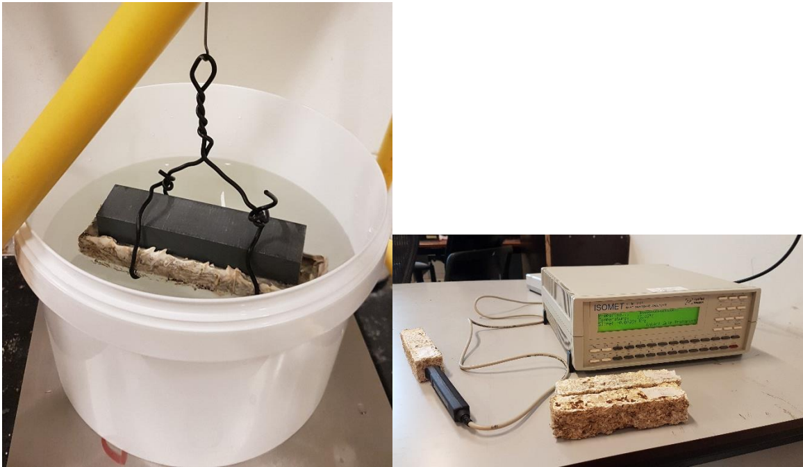
Figure 22 Water absorption test and thermal conductivity test set-up.
