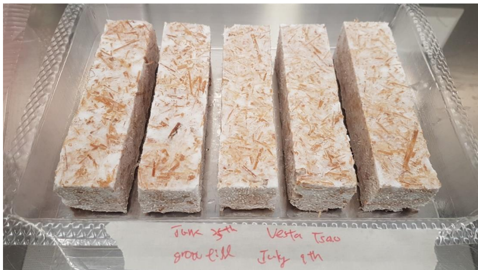
Figure 21 Normal growth samples demolded after 7 days of incubation period and left in the sterilized box for a longer growth.
