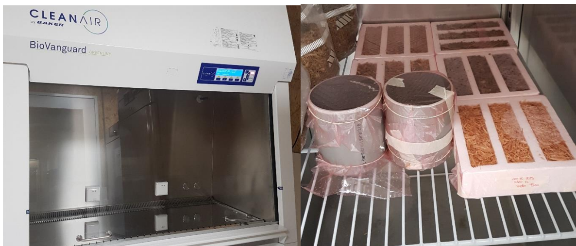
Figure 20 Samples hand-packed in the laminar airflow environment (left) into molds with various substrate ratios and incubated in the growing chamber (right).
