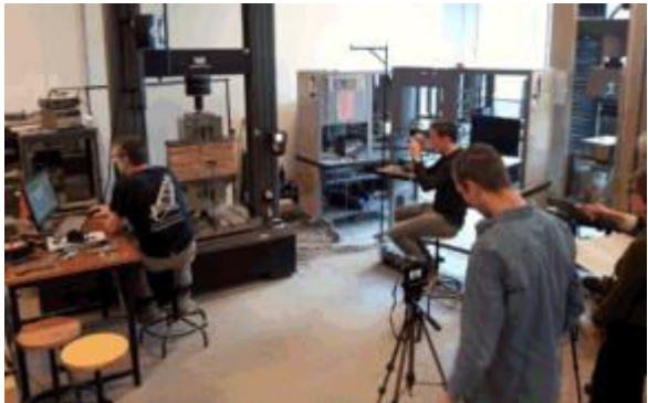
Fig.10. Testing three wall specimen. Intron type 5985
