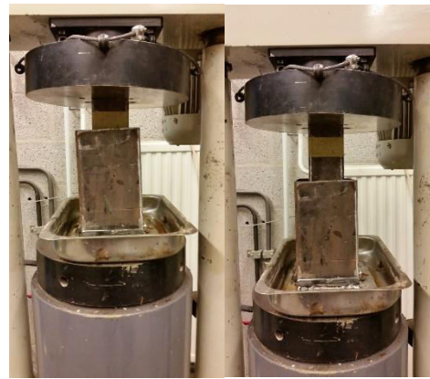
Fig. 4. First compression tests with three types of mycelium specimen in the first loop
