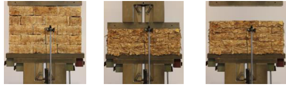
Fig.11. Photos of the test showing the start of loading, at maximum load, and after elastic behaviour
