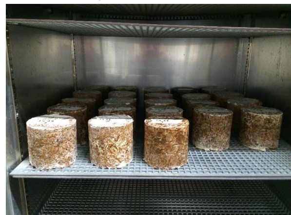
Fig. 5. Drying the test samples, different labelled categories present the different variants
