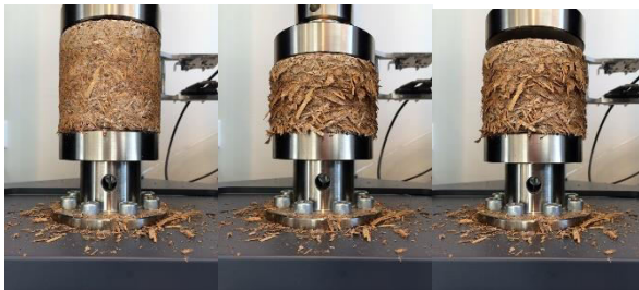
Fig.6. Photos showing the start of loading, the maximum load, and the same specimen after elastic behaviour
