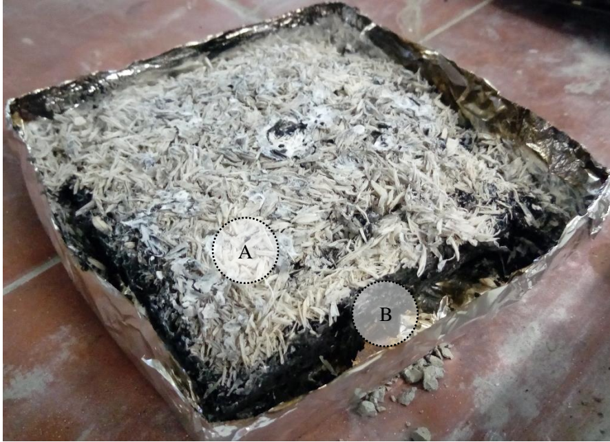
Figure 9: Decomposed mycelium composite with A: silica-ash layer on the heat exposed surface and B: carbonaceous char through the composite core and on the unexposed surface.
