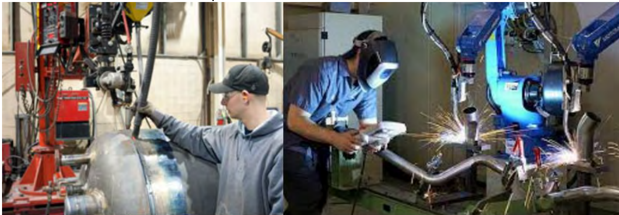
Figure 17: Manually place the weld wire into the joint(left) and teach the robot start from the proper position(right) [HUB21]
