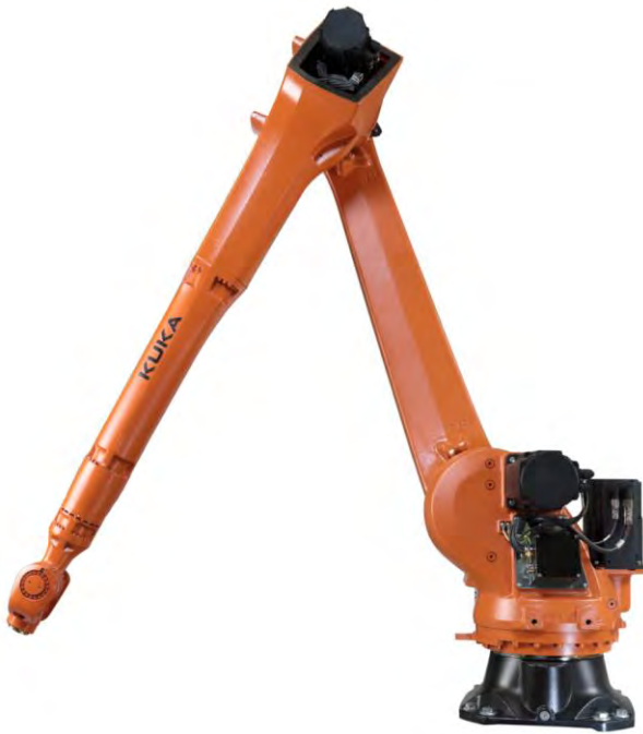
KUKA. Ref. KR 20 R3100 Max. Reach: 3101mm. Weight: 549kg
