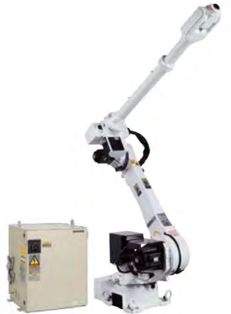
PANASONIC. Ref. GIII-HH020L Max. Reach: 3281mm. Weight: 535kg
