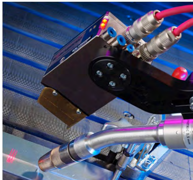
Figure 19: Laser sensing principle diagram (left) and optical seam tracking sensors (right) [HUB21]
