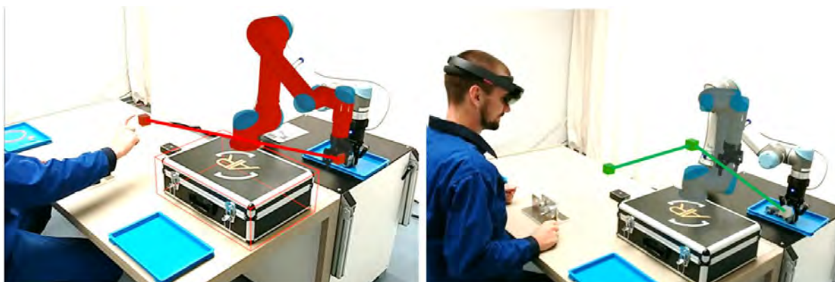
Figure 15: VR application in the robot pose-estimation. User highlights possible collision (left). Robot finds new path (right)
