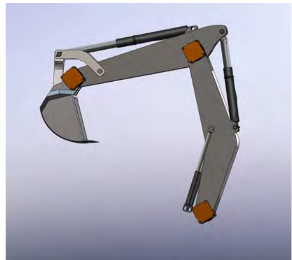
Figure 14: An electric actuator at each joint and a hydraulic actuator piston between two links model
