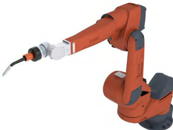
CLOOS. Ref. QRH-390-E Max. Reach: 3015mm. Weight: 350kg
