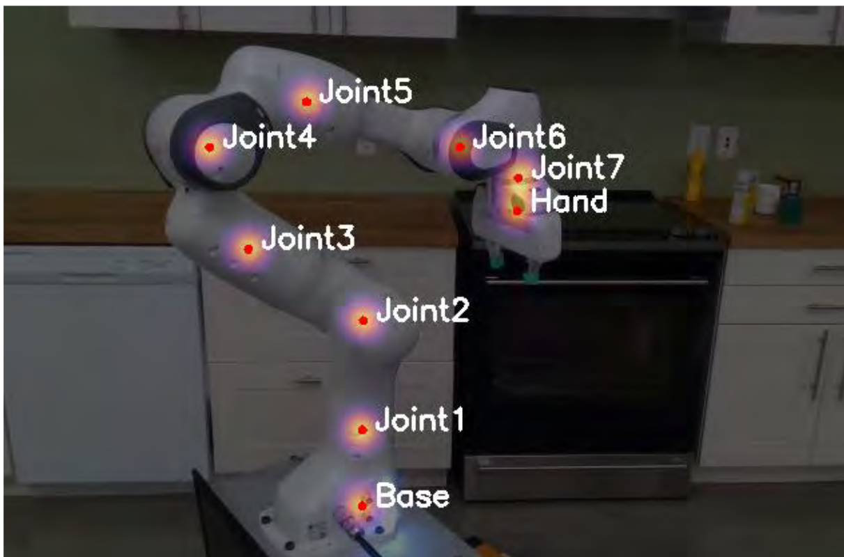
Figure 12: DNN technology applied on robot pose estimation [LEE19]
