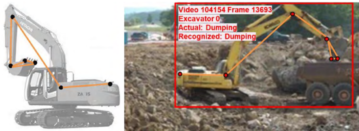
Figure 14: Application of surveillance camera and IMU sensors for the pose estimation of articulated machines [LUO21]
