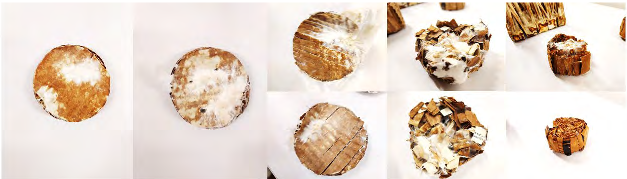
Figure 9: Cardboard samples starting at the left with the control, the vertical holes, the alternating direction strips, the abstract chunk, and the vertical assembled substrates.
