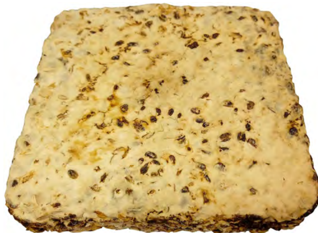
Figure 1. Representative mycelium ( T. versicolor ) – wheat grain composite grown for 18 d and dried at 50 °C for 48 h.
