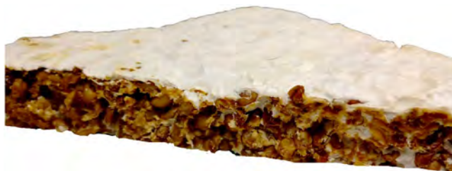
Figure 7. Cross section of the mycelium-wheat composite showing the differences in hyphal density at the surface and the core.
